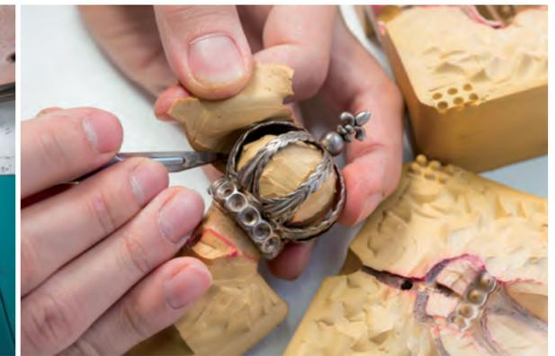
Production of rubber mould using a so-called relief cut
