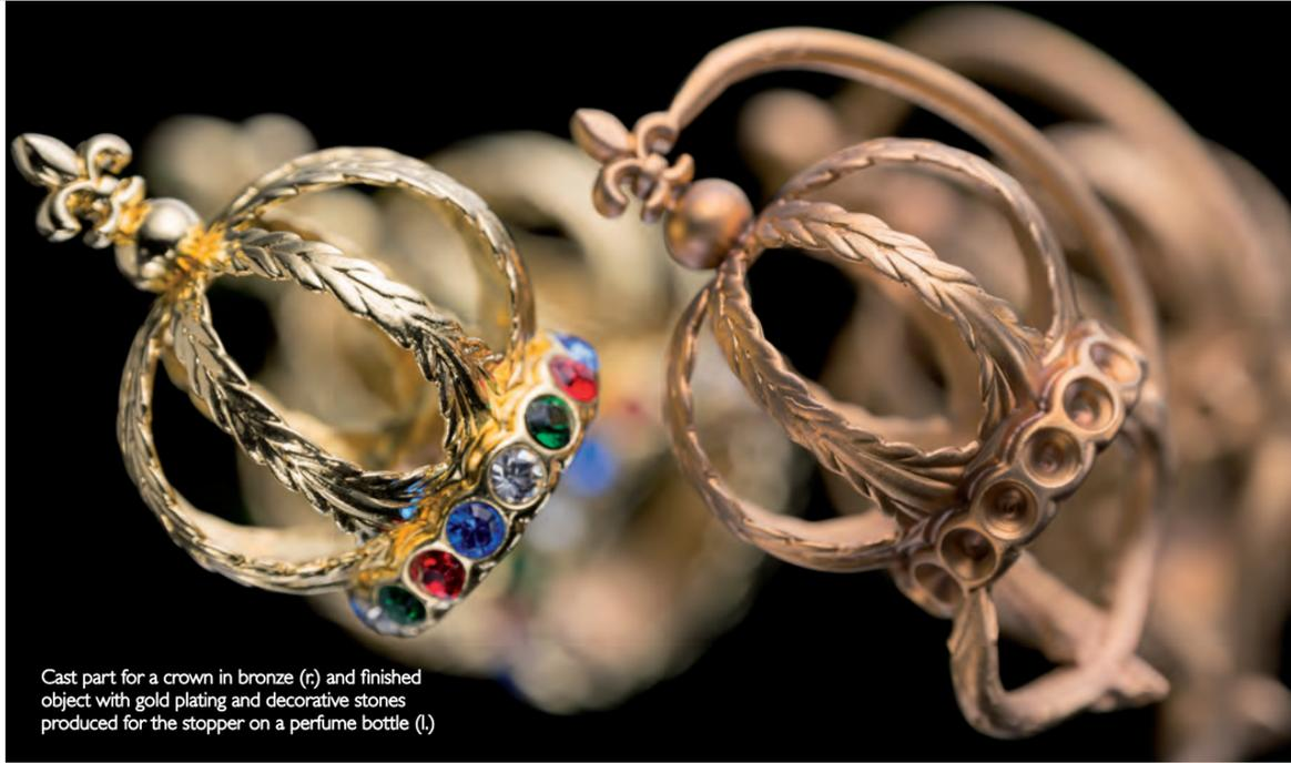
Cast part for a crown in bronze (r) and finished object with gold plating and decorative stones produced for the stopper on a perfume bottle (l.)
