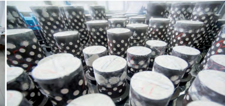
The wax trees are then placed in cuvettes and embossed in a chalky mass
