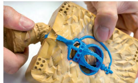
To retrieve the wax component undamaged from the mould, the spiral-shaped rubber is carefully pulled out
