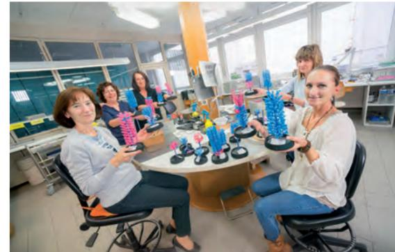
During the fitting stage, the wax components are carefully put together to form wax trees
